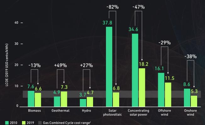
LCOE range for combined cycle gas turbine power generation, which is the typical technology used in gas power stations. Sources: IRENA Renewable Copyright, Lazard's Levelized Cost of Energy Analysis
